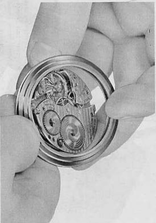
Figure 53 — Hamilton Pocket Watch — Case Screws Removed
