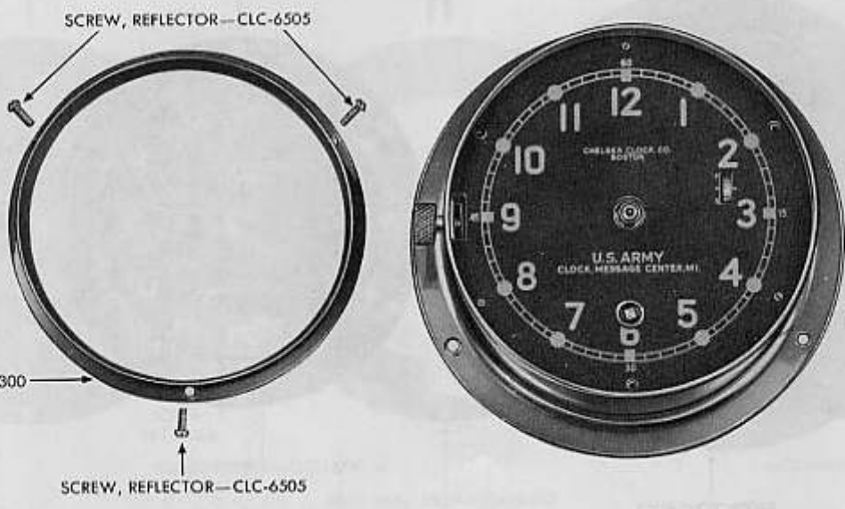
Figure 205 — Message Center Clock M1 — Reflector Removed
