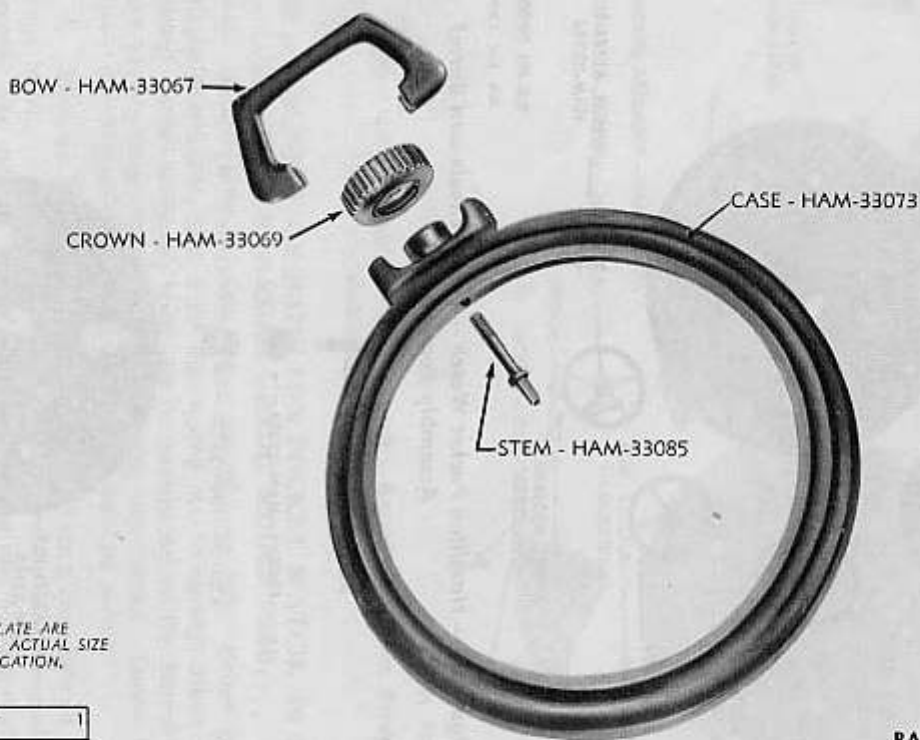
Figure 67 — Hamilton Pocket Watch — Case With Bow, Crown, and Stem Removed
